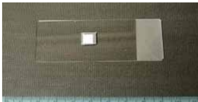
Fig.2. Photograph of silver substrate (5×5mm) mounted on slide glass prepared by gas deposition method.
