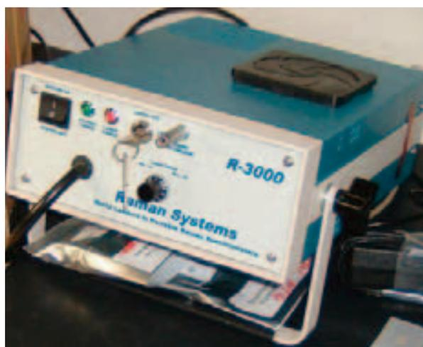
Fig.2. The Raman Systems R-3000, with 785 nm solid-state diode laser, a fiber optic probe, has a wavelength range of 200-2700 cm<sup>-1</sup>(laser resolution:10 cm<sup>-1</sup>).
