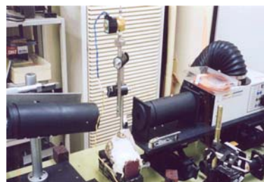
Fig.2. The PCS particle analyzer system used to measure the velocity for bombarded particles.
