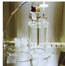
Fig.1. The particle gun device for the delivery into plant cells of plasmid DNA coated on particles driven by gas pressure
